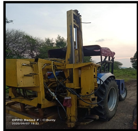
Preparation of Post driving machine
